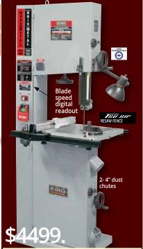
Comes with: a 1/2" x 6 TPI wood cutting blade, 1/2" x 10 TPI metal cutting blade, laser guide, work lamp, miter gauge and a precision "TRU-RIP" aluminum rip fence with resaw guide
